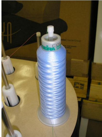
Pic. 9: Seating the Thread Cone on the Thread Tree Tray and Adjusting the Thread Guide Tip to the Height of the Thread Cone
